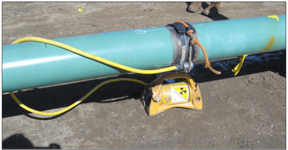
Figure 3: Industrial Radiography Device Using Iridium-192
